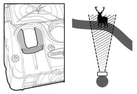
Push the Zone Control shutter up for centered detection.
