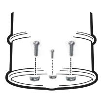
Slide feeder over three **Bolts** that are sticking firmly through the bottom of the drum. Attach **Feeder Kit** to the **Drum** using the three provided **Wing-Nuts**.
