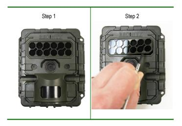
The windows covering the IR Array, lens, WalkTest indicator and light meter may all be cleaned with glass cleaner or water using a soft non-abrasive cloth.
