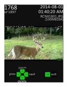
Play Videos – When you select this option, the camera will enter into a slide show function to view thumbnails of the videos on the memory card. The LEFT and RIGHT directional buttons will allow you to scroll through the thumbnails. The UP directional button will play the video while the DOWN directional button will allow you to delete the video being viewed at that time. Pressing the OK button will allow you to exit from the video slide show and return you to the Home page.
