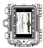
This camera can be powered by a rechargeable lithium battery pack LIT-09/LIT-C-8 (sold separately). This type of battery is less affected by cold temperatures and lasts up to 2 times longer than alkaline batteries.
