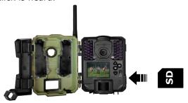
We strongly suggest to slow format the SD card on a computer before use, even more if it has been used in another device. This will maximize the memory card capacity and compatibility.
